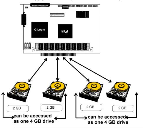
Spanning for RAID 10, RAID 30, or RAID 50
